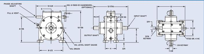
One Rotation of Adjustment Shaft, while running or stopped, provides approximately 51/2° Radial Movement of Output Shaft (66:66:1 Ratio)
