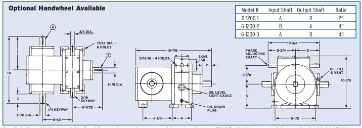
One Rotation of Adjustment Shaft, while running or stopped, provides approximately 5½° Radial Movement of Output Shaft (66:66:1 Ratio)
