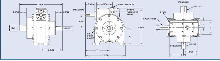
One Rotation of Adjustment Shaft, while running or stopped, provides approximately 51/2° Radial Movement of Output Shaft (66:66:1 Ratio)
