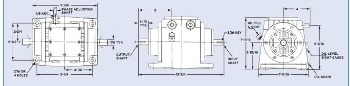
One Rotation of Adjustment Shaft, while running or stopped, provides approximately 3<sup>3</sup>/4° Radial Movement of Output Shaft (96:1 Ratio)
